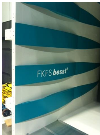
Fig. 3-3: Detailed view of flow guiding elements (FKFS besst ® )
